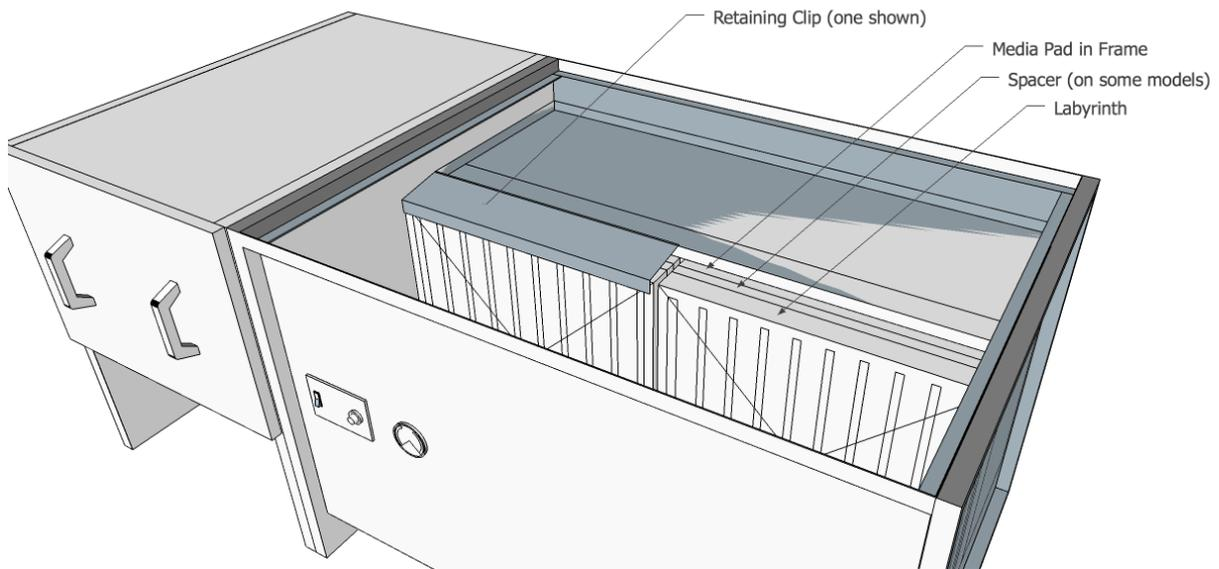
The main filter is accessed via the door on the filter housing (to the left of the main unit). This can be opened by rotating the quarter turn latch and swinging the door forward. Once the door is open, a clamp bar is exposed which holds the filter in position against soft rubber seals. The clamp bar can be loosened, allowing the main filter to rotate forwards and be removed as per the following diagram.
